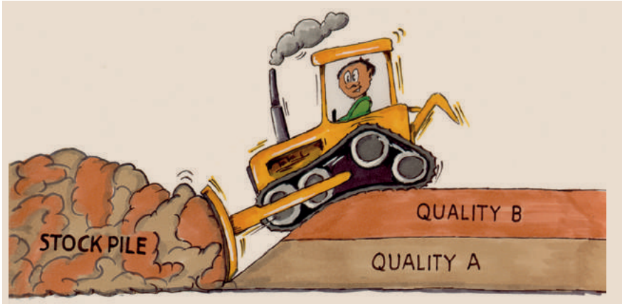
Figure 18-13: Not recommended method for blending in borrow pit Source: SADC Guideline (2003).
