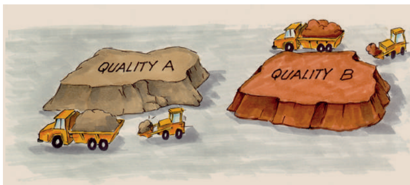
Figure 18-14: Loading from two separate stockpiles in the borrow pit
