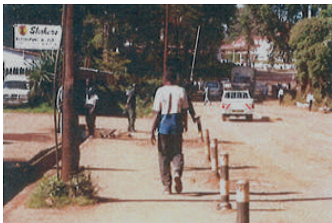
Figure 10-8: Simple poles used to increase safety for pedestrians
