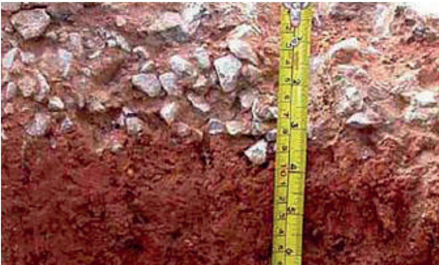
Figure 7-10: Crushed stone armouring on laterite
