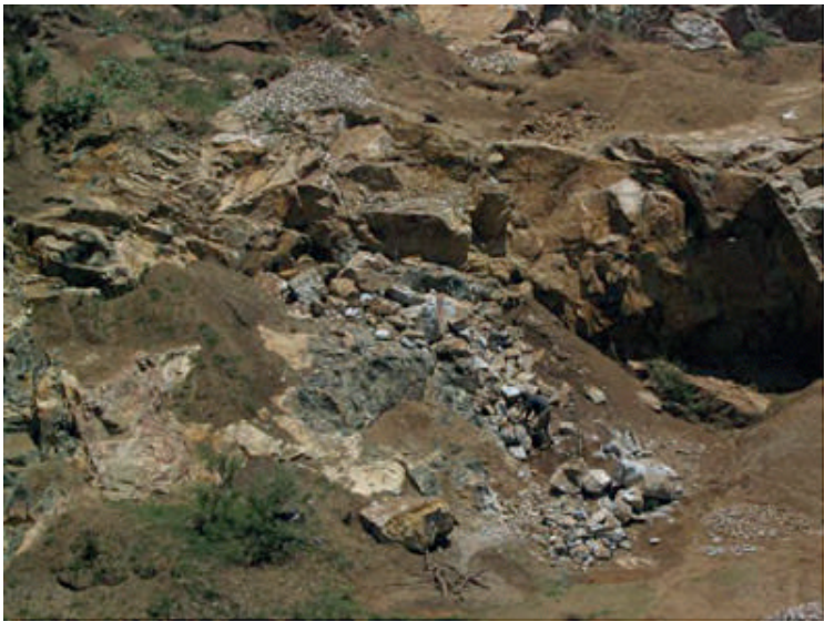
Figure 5-7: Variable weathering in quarry
