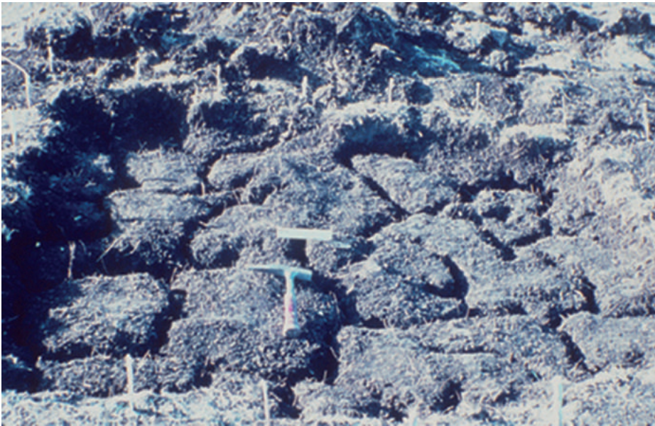
Figure 6-2: Cracking on expansive clay
