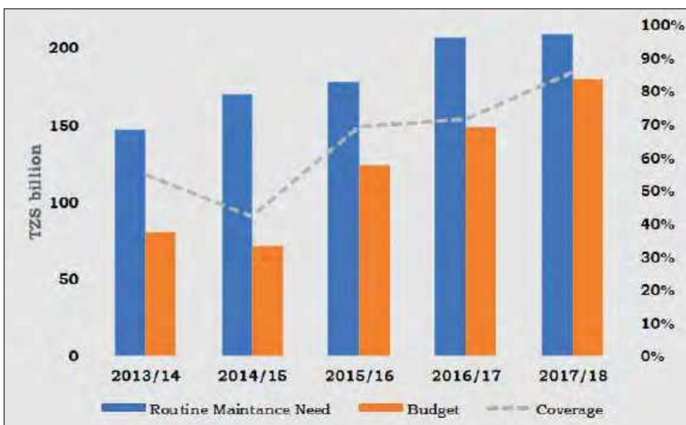
Figure 1.3: Routine Maintenance Needs, Budget and % Coverage
