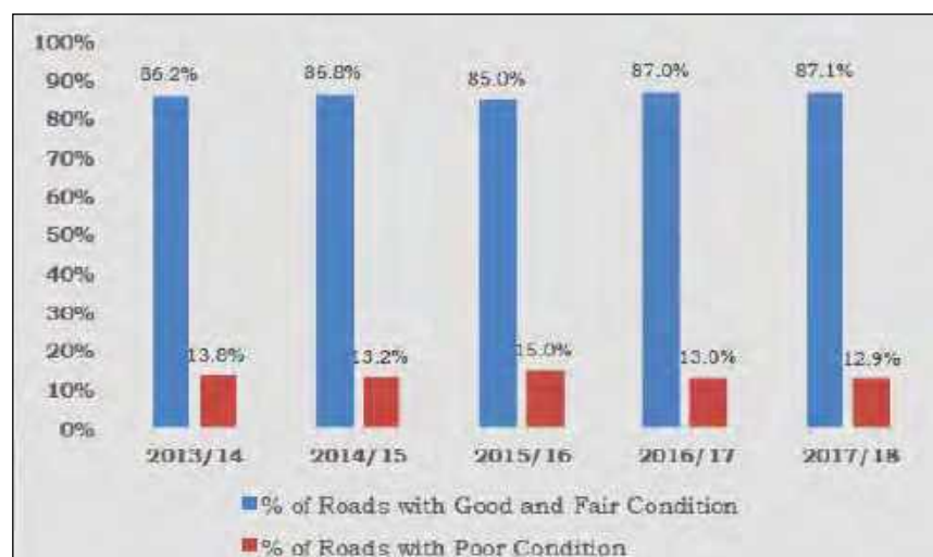
Figure 5.1: Trend of Road Network Condition
